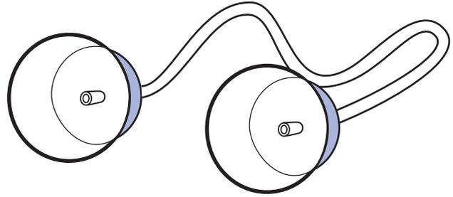
Make a small hole in the bottom of both cups with a nail. Force the tubing into the holes. It should fit very tightly.
