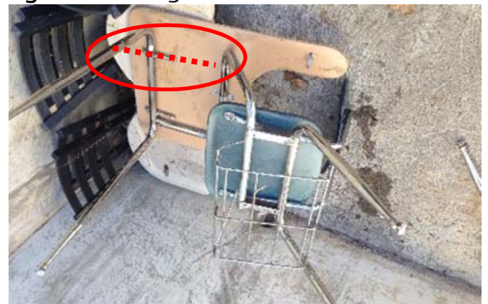
Figure D: Missing cross brace
